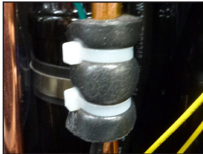
Figure 8: Thermistor attached to the refrigerant line.
